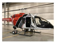
searchlight, night vision capability, rescue hoist, and a 180-gallon water tank, making it multimission capable. The aircraft is also equipped with upgraded safety features, including energy crash attenuating seats with 4-point harnesses, rupture-resistant fuel tanks, and a cutting-edge protection system to mitigate the risks of wire strikes while flying at low altitudes.
